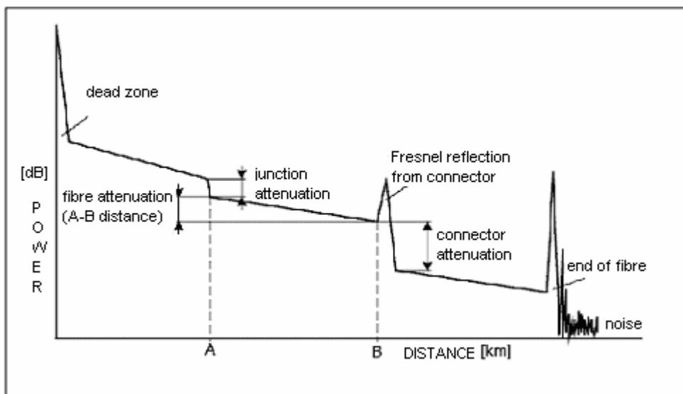
Fig. 5. Reflectogram of the examined length.
