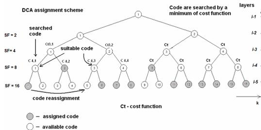
Fig. 3. DCA assignment scheme.
