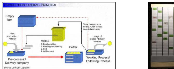
Fig. 1. Transportation Kanban Process[1] and "Sm@rt Logistics" Singlearea-eKanban Board
