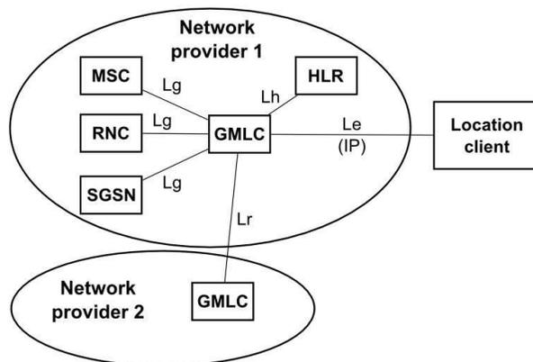
Fig. 1. Architecture of location system.
