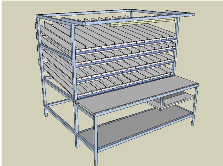
Fig. 3. D drawing of Pick By Light
