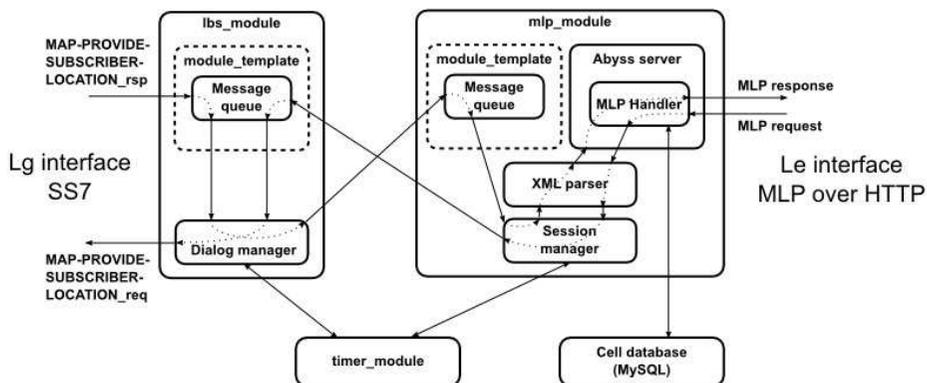
Fig 2. Scheme of lbs\_module and mlp\_module.
