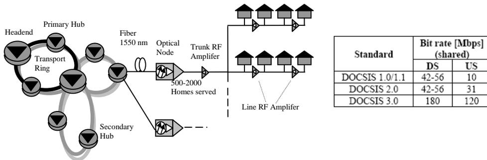
Fig. 4. Architecture HFC network
