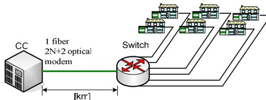
Fig. 2. Active Optical Network
