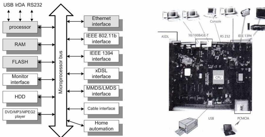
**Fig. 4.** Compact hardware architecture.
