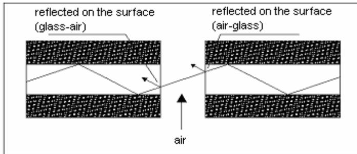
Fig. 2. Phenomenon of Fresnel's reflection.
