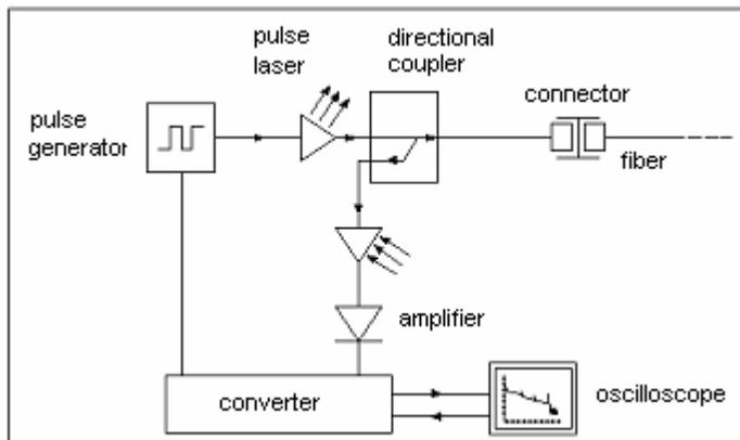
Fig. 3. Diagram of reflectometer.
