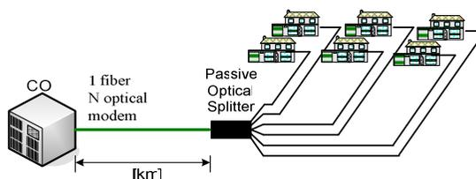
Fig. 3. Passive Optical Network
