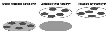
Fig. 4. Frequency spectrum planning
