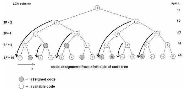
Fig. 2. LCA assignment scheme.
