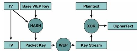
Fig. 2. Per-packet keying operation.
