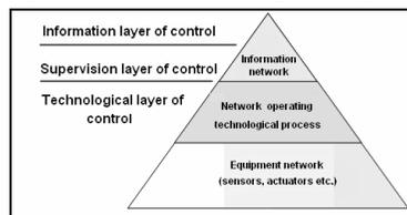
Fig. 1. Hierarchical model of the distributed system of control
