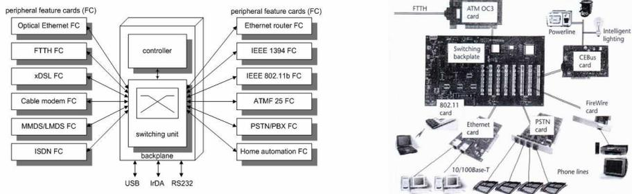
Fig. 3. Modular hardware architecture.
