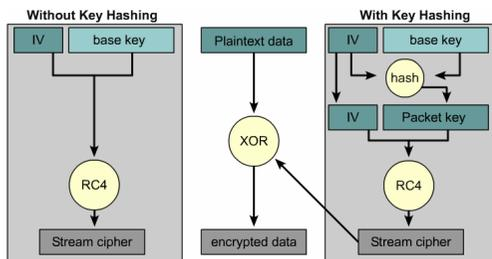
Fig. 1. Temporal key integrity protocol (TKIP).
