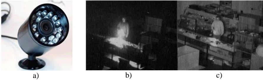
Fig. 1 a) IR illuminated camera, b) Scene without IR, c) Scene with IR
