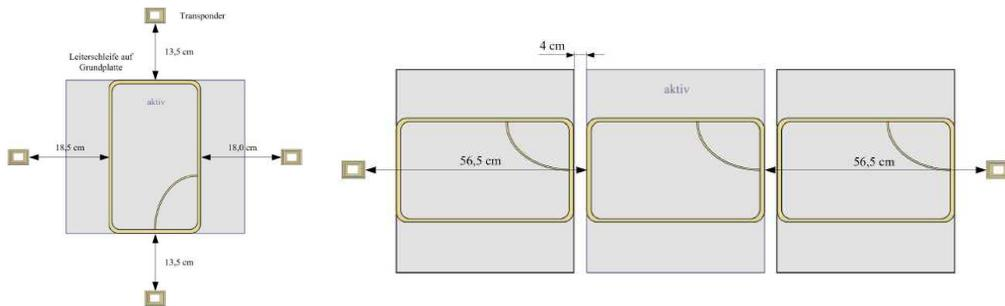
Fig. 4. Maximum transponder identification range of a single and three antenna areas
