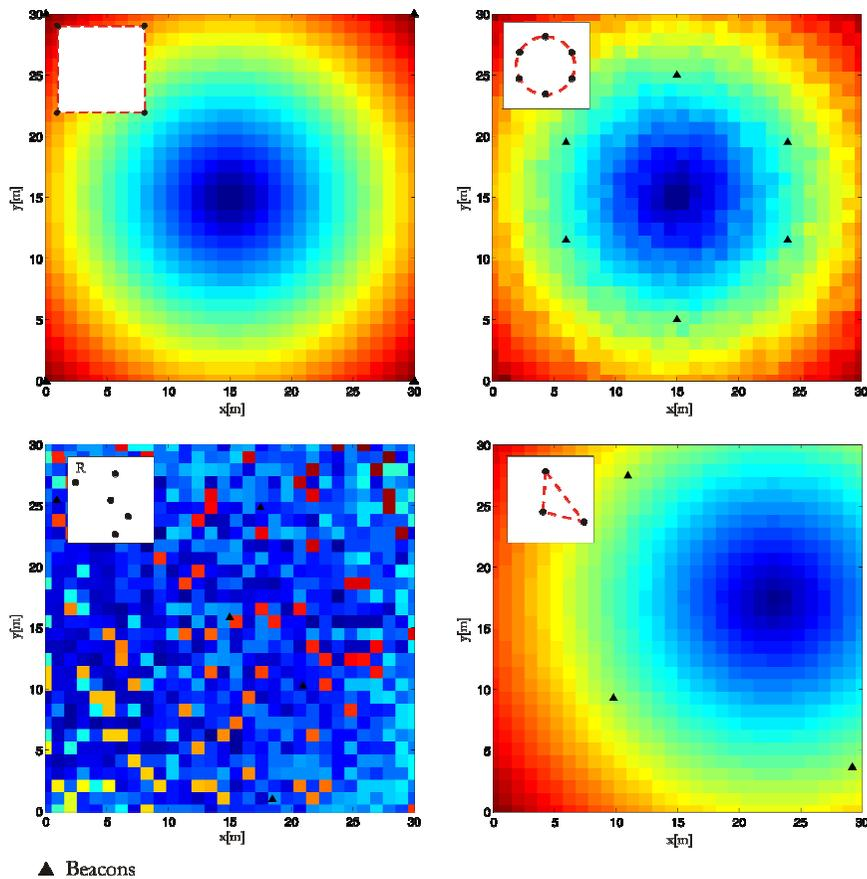
Fig. 2. Figures show RMSE dependency on the beacons topology for DM. The color tone of square element represents the RMSE value in choice point.
